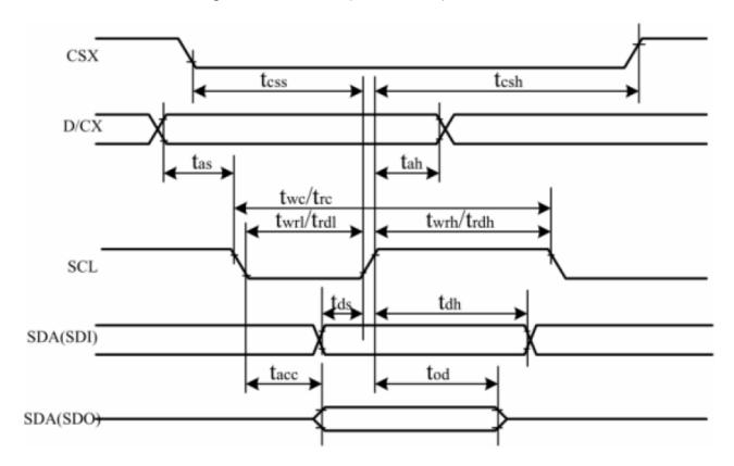
Figure: 4-line series Interface Timing Characteristics
