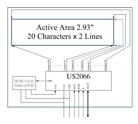
Pins connected to MCU interface: D/C#, R/W#, E, and D0~D7
